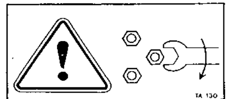
7. ENSURE THAT NUTS ARE KEPT TIGHT
